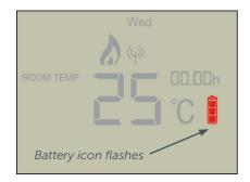
The thermostat will inform you when the batteries need to be replaced by displaying the battery icon on screen.
